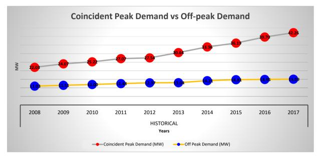
In 2013, there was a substantial increase of demand of 11.245% due to the installation and operation of our 1-10MVA unit in the area of mallig region were large load consumers are present in the areas such as industrial rice mills and commercial establishment in the area, voltage imbalance was also address in the area.
